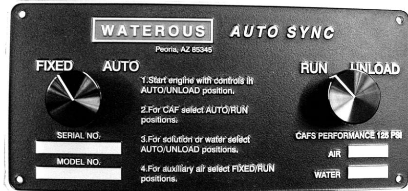
Figure 2 Manual Auto-sync panel
